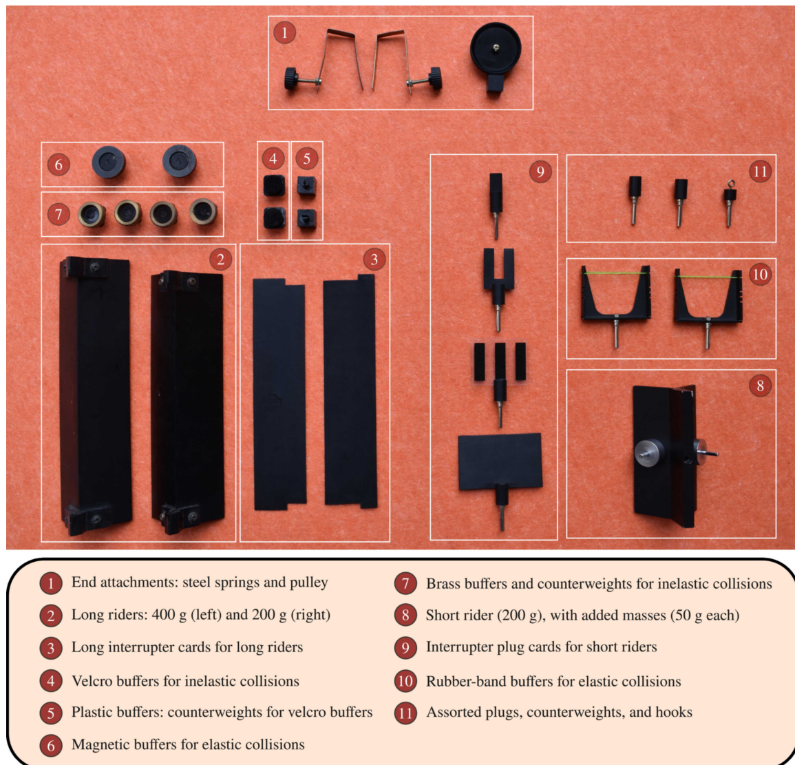
Figure 2.2: Accessories for the air track. The end attachments are placed at either end of the track. The remaining accessories are placed on one of the two different types of riders, long or short. The long riders come in two types: the heavier 400 g rider is slightly longer than the 200 g rider. On the left are all the attachments for the long riders, and on the right are all the attachments for the short riders.
